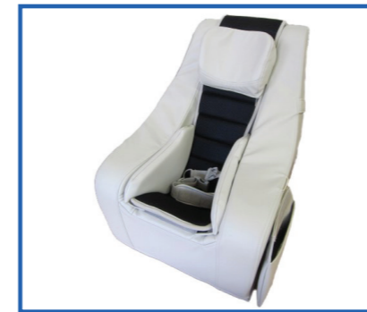
Side filler pads, Laterally velcroable The seat width can be adjusted by attaching it to the inner wall of the chair. The thickness is 30 mm and the inner padding consists of three 10 mm thick panels so that it can be adjusted in 10 mm increments on each side.
